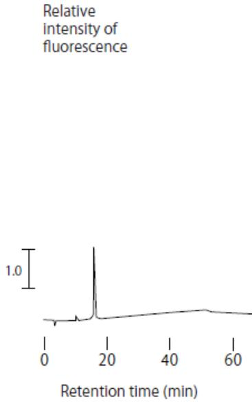
Column : PALPAK Type R (4.6 mm $\Phi$  × 250 mm)
