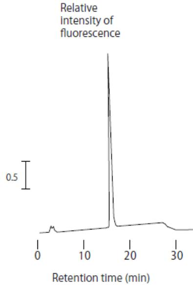
Column : PALPAK Type S (4.6 mm $\Phi$  × 250 mm)
